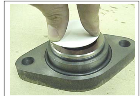
Figure 19, Stationary set install
